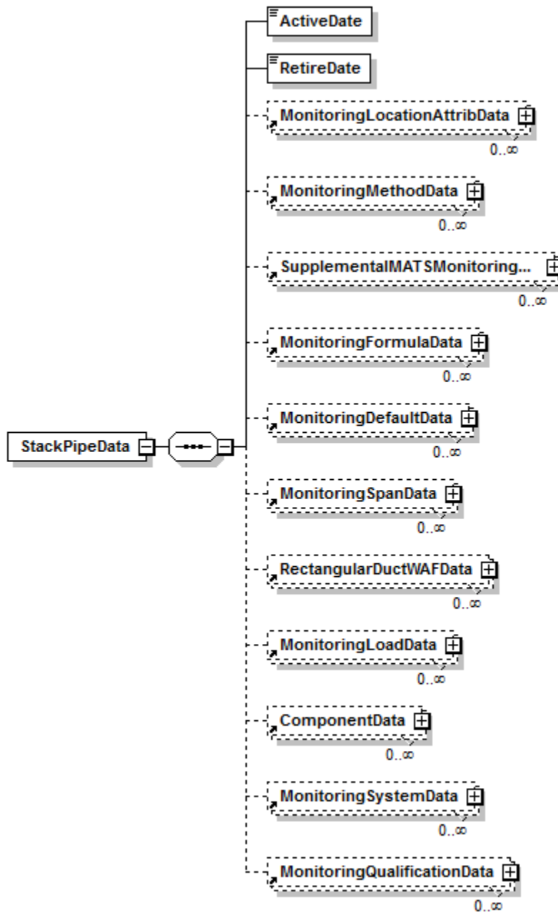
Figure 6: Stack Pipe Data Elements
